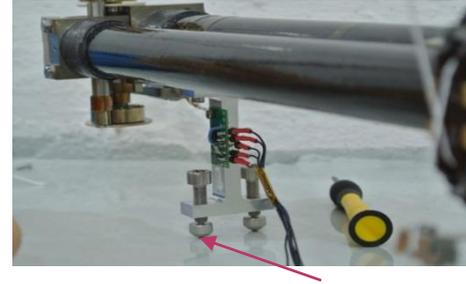
Test performed on the epoxy floor, using Miniature Ball Transfer Units (BTU)- 0g facility
