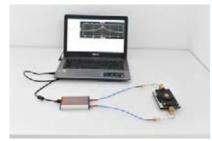
QWED SPDR and Q-Meter™ setup for dielectric material measurements at 5GHz
