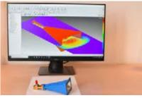
Pyramidal horn antenna designed with QuickWave™ software against its computer model
