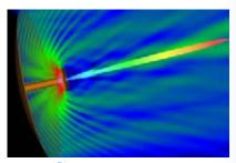
QuickWave<sup>™</sup> design of double reflector antenna for SATCOM applications.
